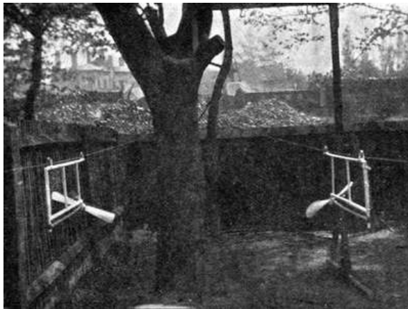
FIG. 35.—PROPELLER TESTING. Showing distance separating the two wires.
