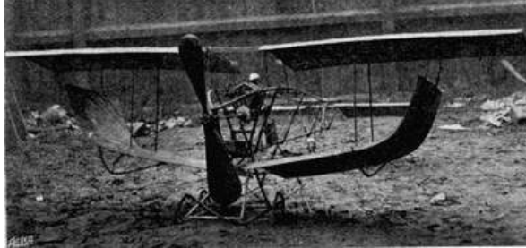
FIG. 19.—MR. STANGER'S PETROL-DRIVEN MODEL AEROPLANE. [Illustrations by permission from electros supplied by the "Aero."]
