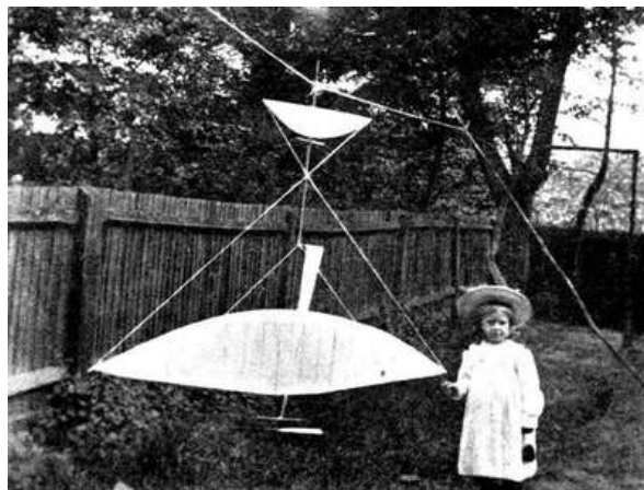
FIG. 10.—LARGE MODEL MONOPLANE. Designed and constructed by the author, with vertical fin (no dihedral angle). With a larger and more efficient propeller than the one here shown some excellent flights were obtained. Constructed of bamboo and nainsook. Stayed with steel wire.
