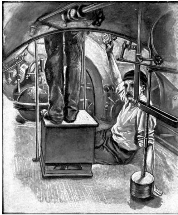
An interior view of the "Holland." The large pendulum on the right actuates mechanism to keep the Submarine at the required depth below the surface.
