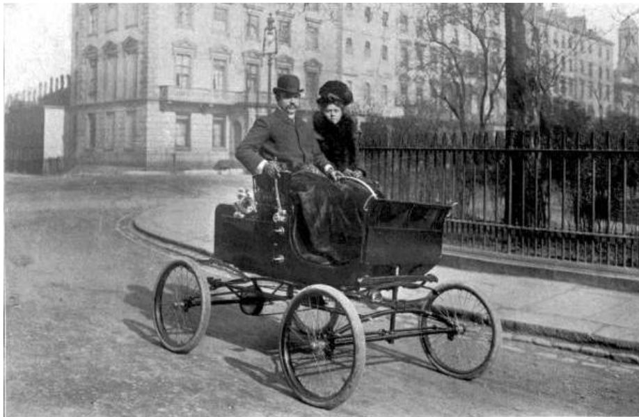
By kind permission of The Liquid Air Co. This graceful little motor-car is driven by Liquid Air. It makes absolutely no smell or noise.
