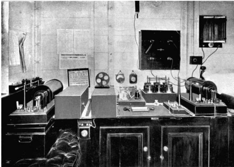
A Corner of M. Marconi's cabin on board S.S. "Minneapolis," showing instruments used in Wireless Telegraphy.
