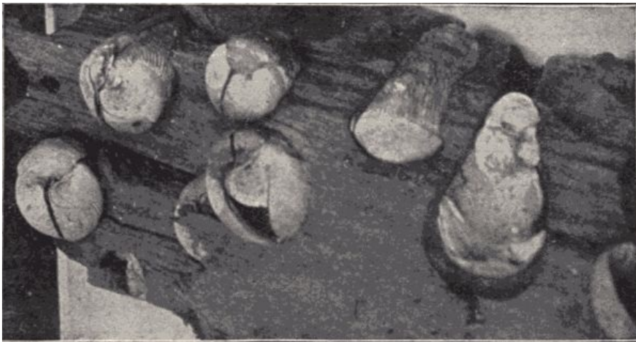
FIG. 107.— Martesias xylophaga , a Pholad, in Panama mahogany. (Photograph by C. H. Snow; permission of Amer. Soc. Civil Engineers.)
