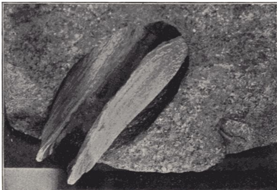
FIG. 105.— Dactylus sp., a mollusc, excavating granite. (Photograph by C. H. Snow; permission of Amer. Soc. Civil Engineers.)
