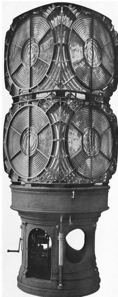
FIG. 54.—FASTNET LIGHTHOUSE—FIRST ORDER SINGLE-FLASHING
