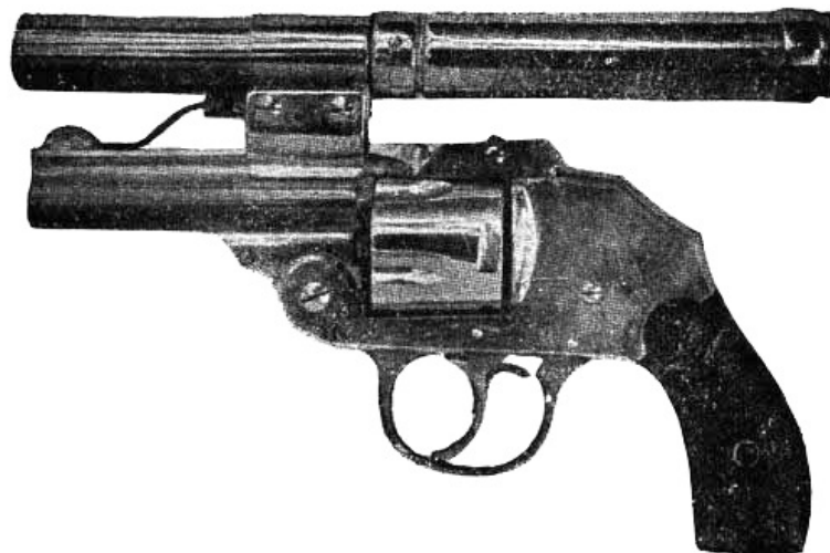
Fig. 63.—The Wespi Searchlight Mounted on a Pocket Revolver.
