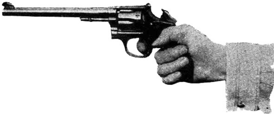
Fig. 84 a.—Showing Thumb when Locking Catch Interferes with Extended Position
