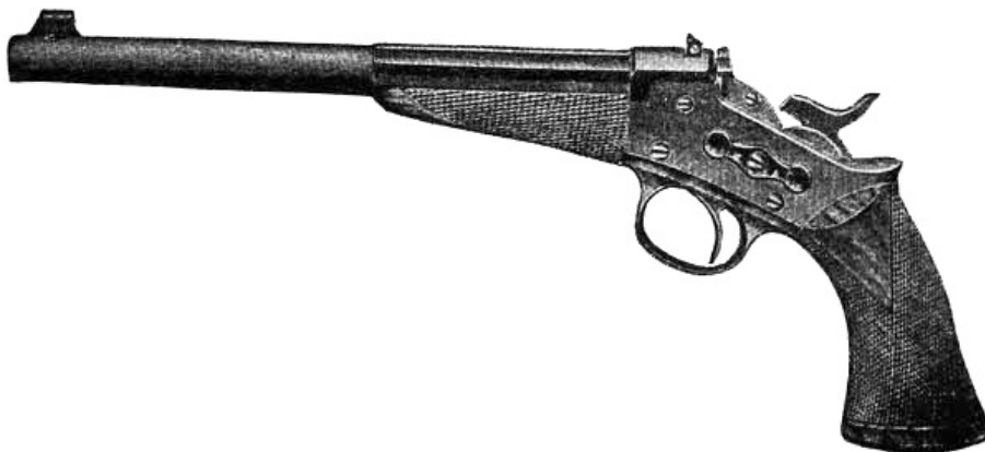
Fig. 15.—REMINGTON PISTOL Ten-inch barrel, weight, 2 lbs., 8 oz.; .44 cal.
