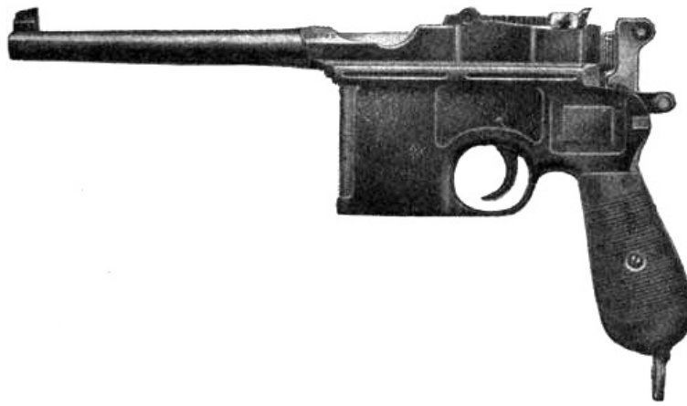
Fig. 12.—MAUSER AUTOMATIC PISTOL Ten shots; 5½ inch barrel; weight, 2 lbs., 7½ oz.; .30 cal.
