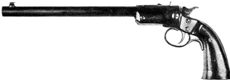
Fig. 14—STEVENS PISTOL, GOULD MODEL Ten-inch barrel; weight, 1 lb., 10 oz.; .22 cal.
