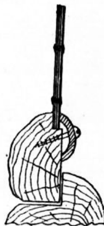
Fig. 187.—Securing Glass to Rustic Casement.
