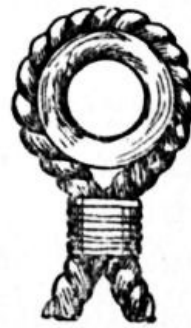
Fig. 110.—Fixing Rope to Eyelet.
