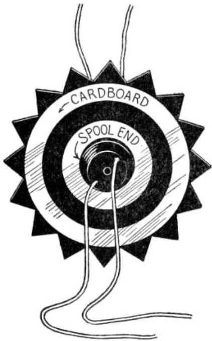
FIG. 111.—Detail of Buzz-saw Whirligig shown in Fig. 108.
