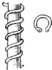
FIG. 1. Probable method of making links for mail.
