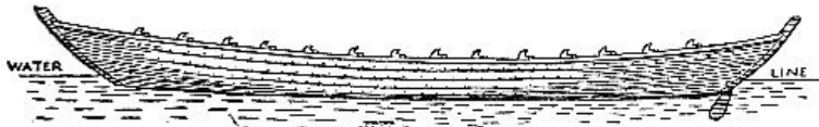
Broadside View of the Nydam Ship now in the Kiel Museum. Observe the horn-like rowlocks and the steer-board
