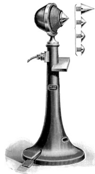
FIG. 126. LARGE ELECTRO-MAGNET. The current is turned on by means of the foot pedal.
