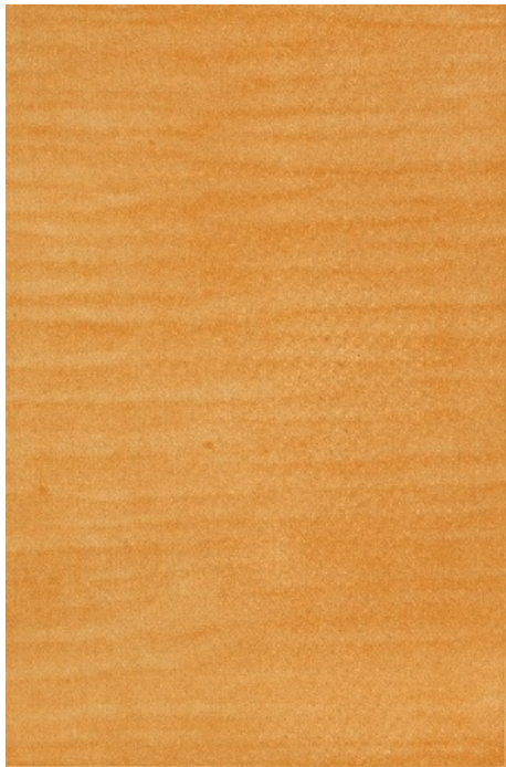
Plate 30. CHERRY MOTTLED IN OIL BEFORE BEING OVERGRAINED.
