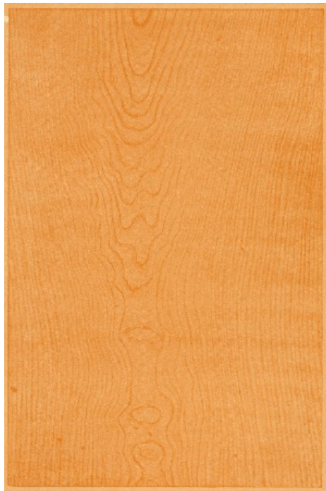
Plate 33. CHERRY MOTTLED AND PENCILLED IN OIL AS FINISHED.
