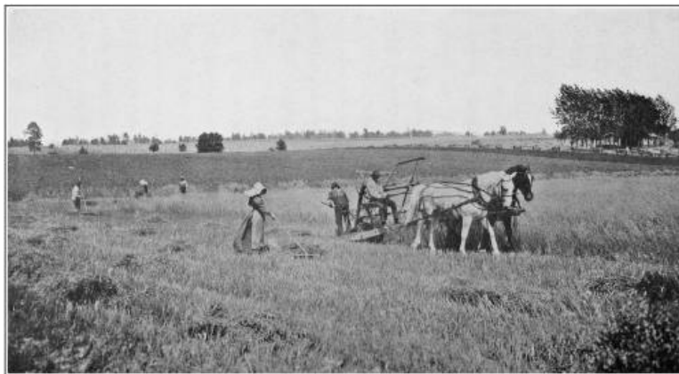
THE McCORMICK REAPER OF 1847, ON WHICH SEATS WERE PLACED FOR THE DRIVER AND THE RAKER
