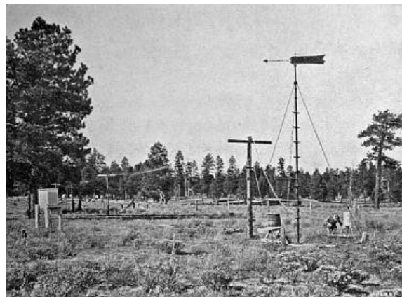
Figure 29. At the Fort Valley Forest Experiment Station, Coconino National Forest, Arizona. A typical meteorological station Forest officer measuring precipitation. Note the shelter which contains thermometers and also the electrically equipped instruments to record the direction and velocity of the wind.
