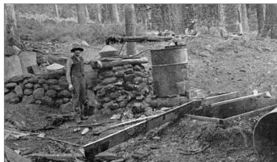
Figure 33. The western pine forests will some day be a great source for naval stores. By distilling the crude resin of the Jeffrey pine a light volatile oil—abietene—is secured which has great healing and curative properties.
