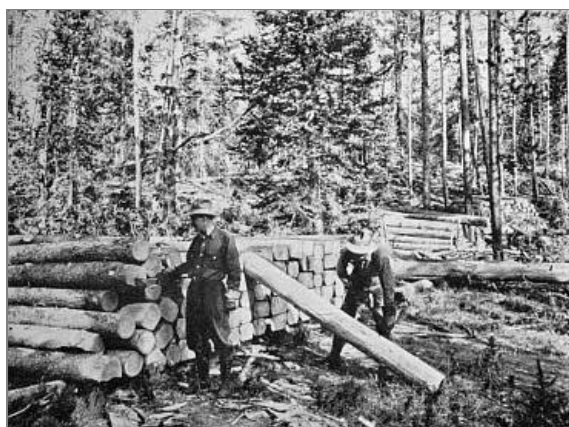
Figure 70. A tie-cutting operation on a National Forest. These piles of railroad ties are being inspected, stamped, and counted by Forest rangers. From this point the ties are
