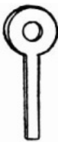
Fig. 4. —The narrow strip extending outward from the ring is pushed through the hole in the upright, and the edge of the leather is fitted into the little grooves just above and below one of the holes ( Fig. 5 ).
