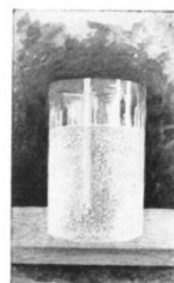
Fig. 9. A glass of cold water on which vapor has condensed in drops.
