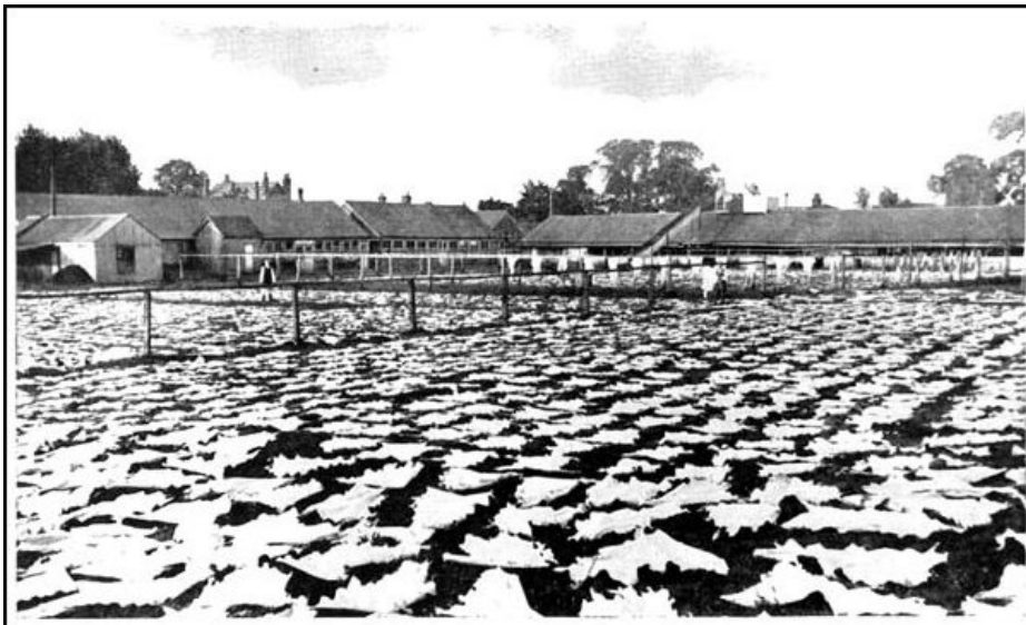
BLEACHING OIL-TANNED LEATHER BY EXPOSURE TO THE SUN The Rosary Leather Mills. Ashtead
