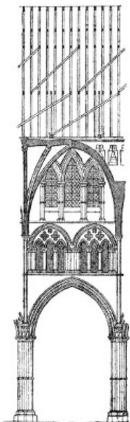
ELEVATION OF ONE BAY ON THE NORTH SIDE OF THE NAVE.
