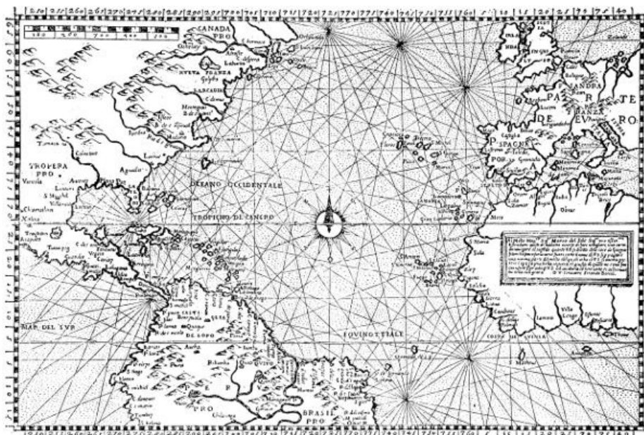
FIG. 3. LOXODROMIC CHART OF NORTH ATLANTIC OCEAN, 1565. A PLAIN CHART WITH LATITUDE DEGREES OF EQUAL LENGTH.
