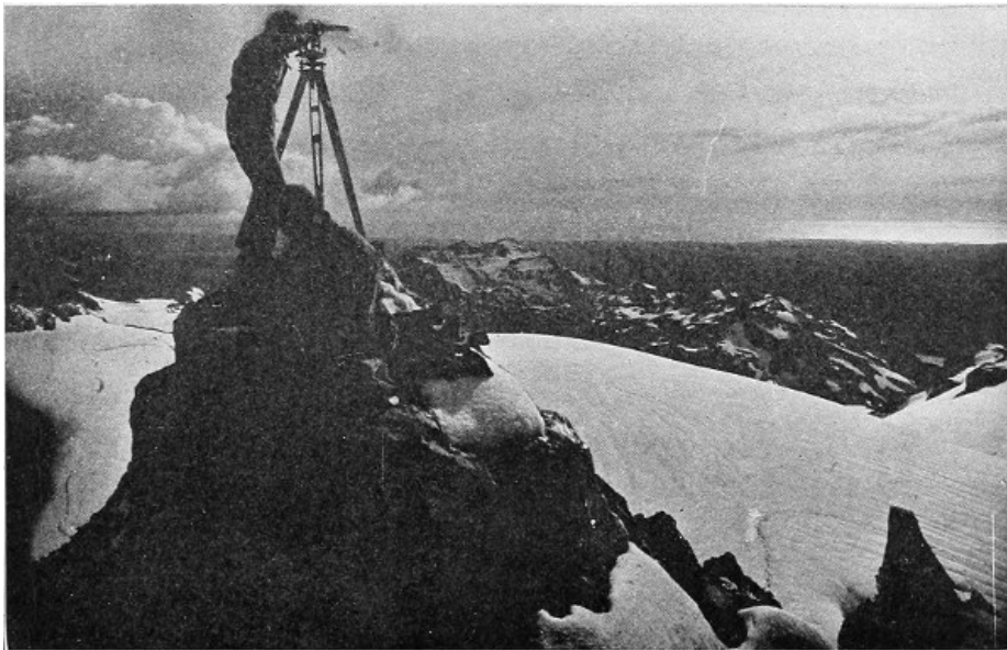
FIG. 10. MEASURING ANGLES WITH THEODOLITE AT TRIANGULATION STATION ON ALASKA COAST.
