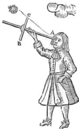
SEVENTEENTH CENTURY MARINER USING A CROSS- STAFF From Seller's "Practical Navigation," London, 1676
