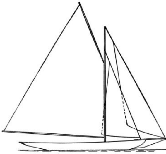
POLE MAST SLOOP
