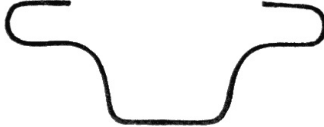
FIG. 4.—SHAPE OF BRASS ROD TO COLLECT THE ELECTRICITY.
