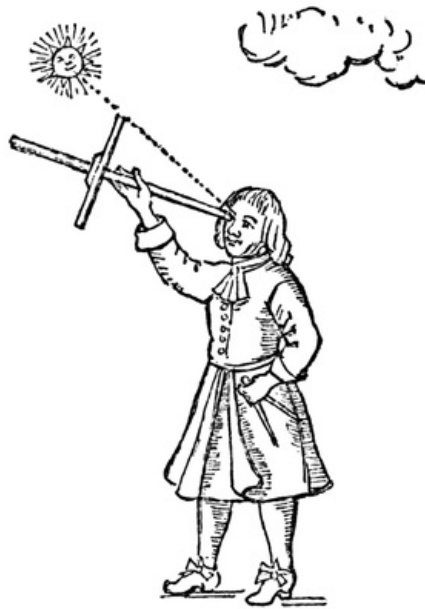
The Figure of the Cross-Staff and the Manner of Observation.
