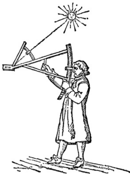
The Figure of the Quadrant and Manner of Observation. (Davis's Quadrant.)
