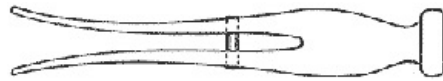
In Attempting to Cut the Hardened Steel Pin the Edge is Drawn Sharp
