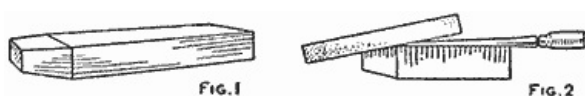
The Sloping Edges on the Block of Wood and the Manner of Whetting a Chisel (Fig. 1, Fig. 2)
