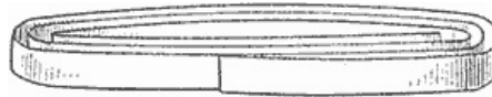
The Filed Edge on the Coiled Metal Retains the Sand Particles as It is Rubbed over the Glass Surface
