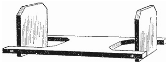
The Ends of the Rack Turn Down, Making a Straight Board
