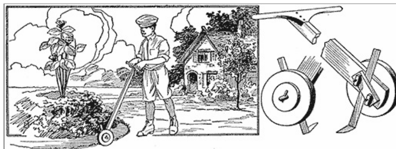
An Edger, Similar to a Garden Plow, for Quickly Trimming the Sod around a Flower Bed
