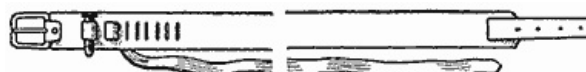
Two Pieces of Leather of Different Widths Forming a Belt for Holding Cartridges
