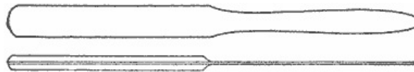
A Palette Knife Made of a Corset Steel and a Wood Handle Attached
