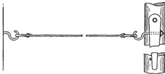
A Lever Attached on One End Post Makes It Easy to Draw the Line Taut
