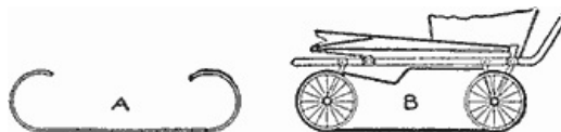
The Runners are Easily Applied to the Wheels of a Go-Cart and Hold Them Solidly
