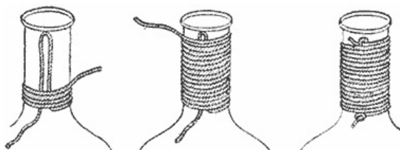
The Ends of the Cord are Held Tightly and the Winding Protects the Hands
