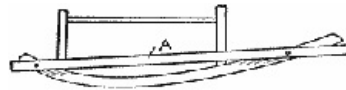
The Strip on the Rocker Prevents the Child Tipping the Chair Too Far Either Way
