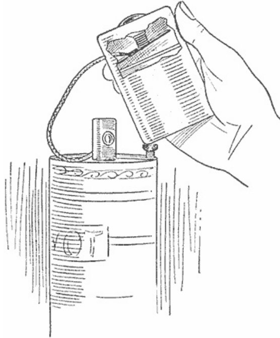
An Instrument Made of an Electrical Pocket Flash Light for Testing Circuits and Instruments
