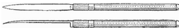
One of the Nibs on the Ruling Pen Sharpened and Used as an Eraser
