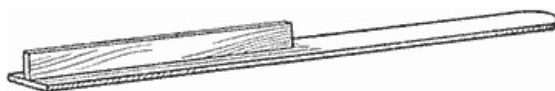
A Flat Surface Strikes the Liquid No Matter Which Way the Stick is Moved
