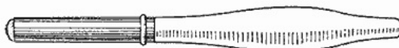
A Small Torch Made of a Penholder is Handy to Use in Soldering Electrical Apparatus
