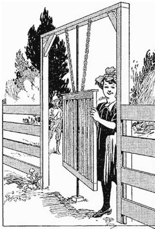
The Gate will Swing in Either Direction and Come to a Rest Where It Closes the Opening
