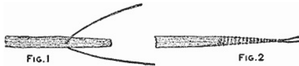
The Wire Prevents the Lace from Raveling and Makes a Tip for Easily Entering the Eyelets (Fig. 1, Fig. 2)
