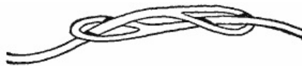
An Endless Thong is Made with Eyes Cut in the Ends of the Leather, and Each Part is Run through the Eye of the Other
