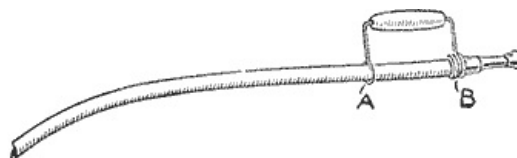
The Handle Is Made of a Piece of Wire and a Package Grip
