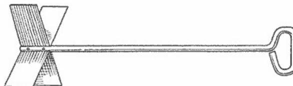
The Chopper Consists of a Rod Handle to Which Blades are Attached by Riveting or Welding
