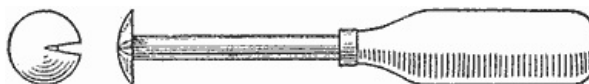
The Shape of the Head Permits a Leverage Action That Lifts the Tack Easily
