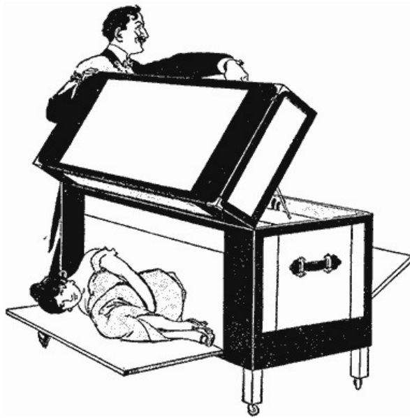
A Shelf and Panel Set at Right Angles to Form a Place at the Back for the Assistant to Conceal Herself, No Matter Which Way the Trunk is Turned to Face the Audience
