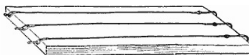
The String is Drawn Taut over the Block, and the Hooks are Caught in the Block End
