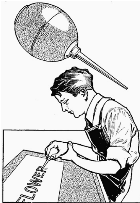
The Oilcan Spout Is the Reservoir to Hold the Paint, and the Bulb Produces the Air Pressure
