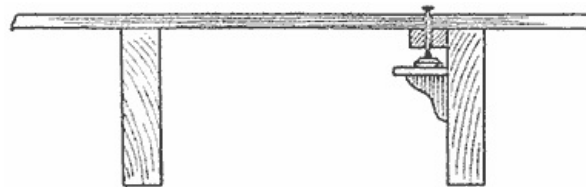
Push Button on Joist
