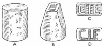
Initials Cut in a Cork Served the Purpose in the Absence of a Rubber Stamp
