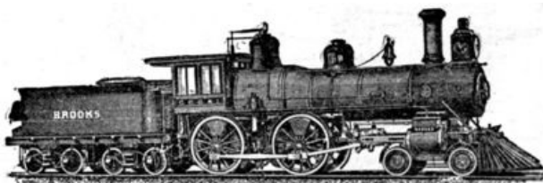
AN AMERICAN LOCOMOTIVE WITH TWO DRIVING WHEELS.
