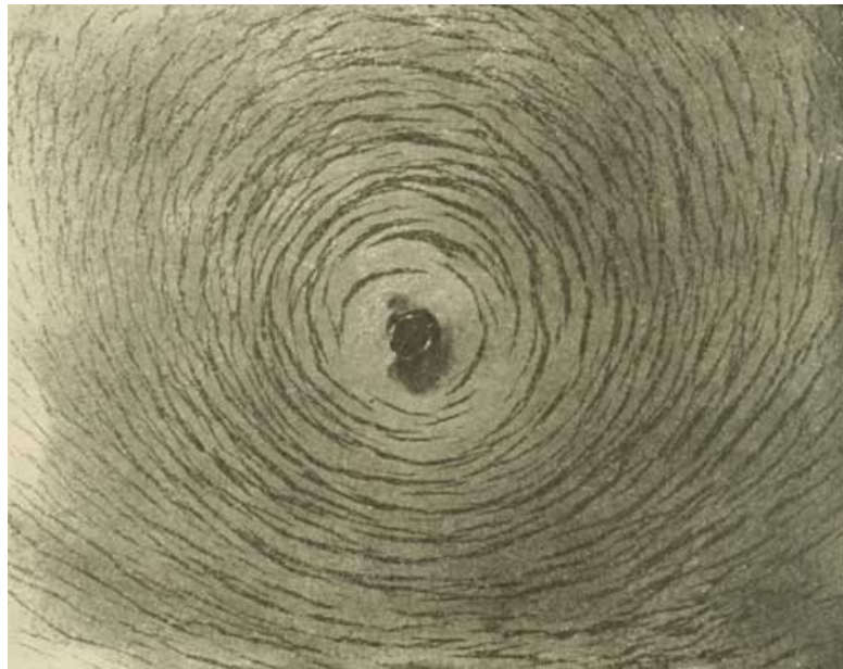
Fig. 4.—Magnetic whirls about the sending wire.
