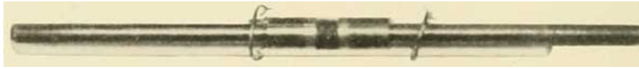
Fig. 6.—The coherer employed to receive the electric waves. (One and a third actual size.)
