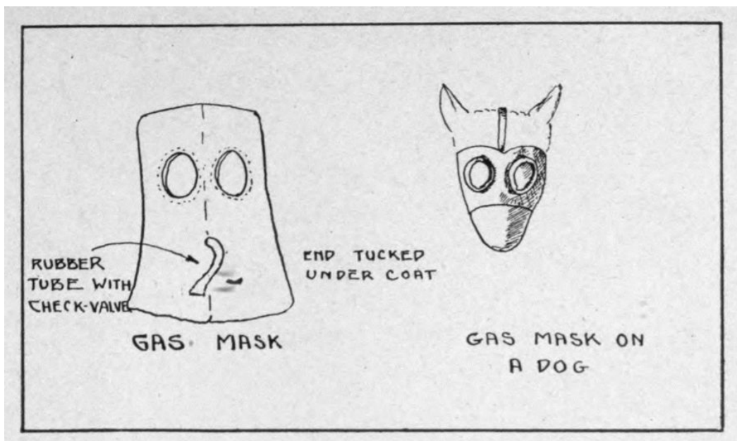
FIGURE 16: Simple gas mask with flutter valve or check valve. Ambulance dogs and horses in the gas zone were equipped as shown.
