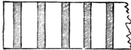
Fig. 29 Wood, with the Strips glued on.
