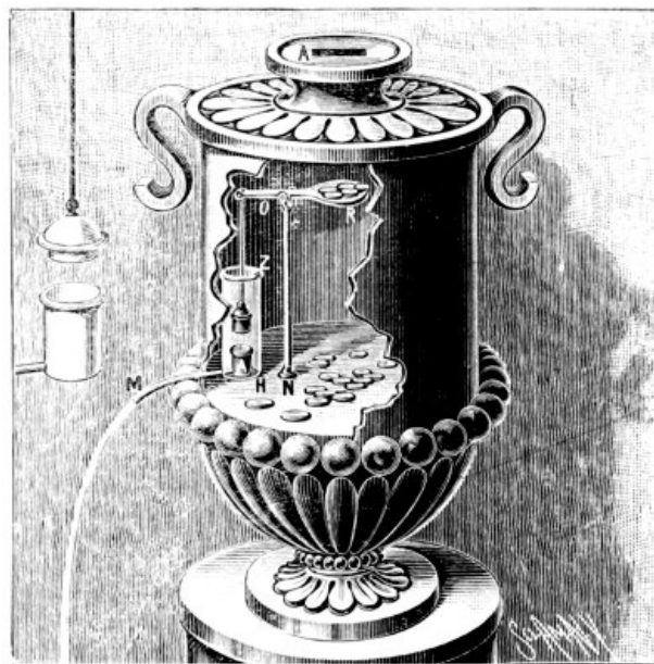
LUSTRAL WATER VESSEL DESCRIBED BY HERON ABOUT 100 B.C.
