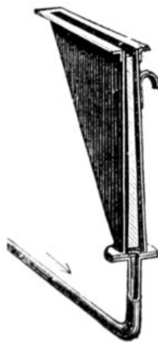
APPARATUS FOR IMITATING THE SMOKE OF A CONFLAGRATION ON THE STAGE OF A THEATER
