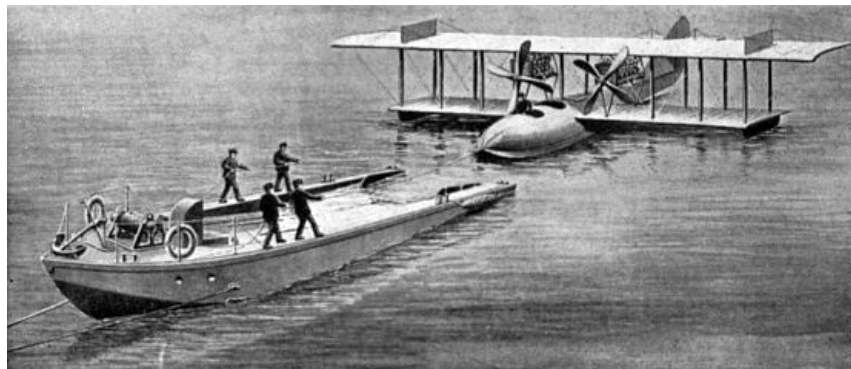
Hauling a Seaplane up on a Barge so that it may be Towed at High Speed by a Destroyer
