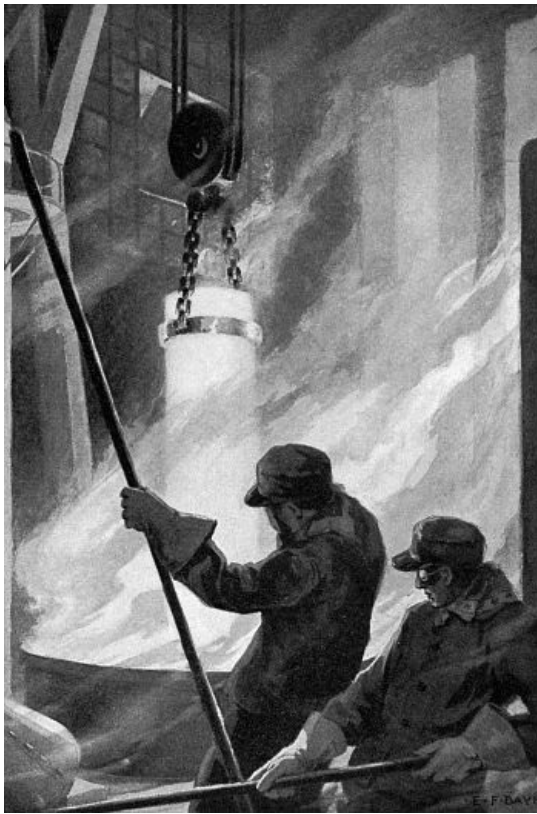
Oil-tempering the lining of a Big Gun (See page 76 )
