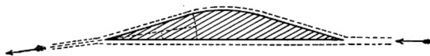
Fig. 48.—The paradox aeroplane that lifts no matter in which direction it is being driven.
