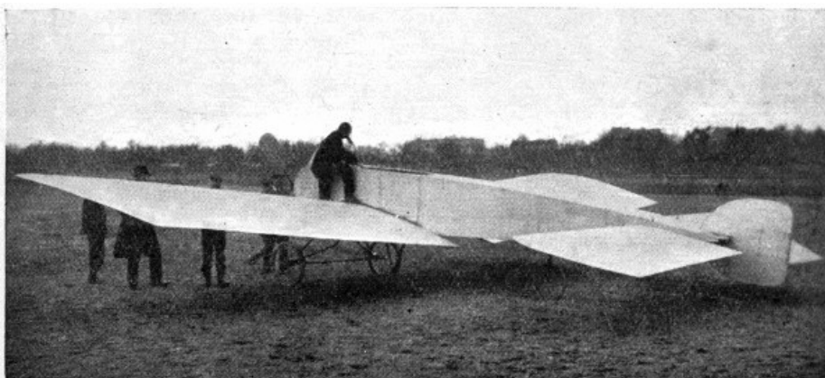
Fig. 71.—Bleriot's machine. This machine raised itself from the ground, but as the centre of gravity was very little, if any, above the centre of lifting effect, it turned completely over in the air.
