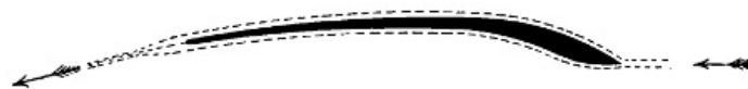
Fig. 88.—The very narrow aeroplanes, or sustainers, employed by Mr. Philipps. It has been supposed that the air in striking at A was deflected in the manner shown, but such is not the case. The air in reality follows the surface, as shown in the dotted line in the second illustration.
