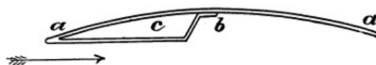
Fig. 30.—Cross-section of condenser tube, made in the form of Philipps' sustainers, in which c is the steam passage.
