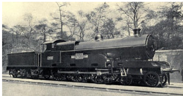
"PATRIOT."—A TYPICAL EXAMPLE OF THE "CLAUGHTON" CLASS OF 6 FEET 6 INCH, SIX WHEELS COUPLED EXPRESS PASSENGER ENGINE WITH SUPERHEATED BOILER; FOUR H.P. CYLINDERS, 15-3/4 INCH BORE × 26 INCH STROKE; BOILER PRESSURE, 175 LBS. PER SQ. INCH; MAXIMUM TRACTIVE FORCE, 24,130 LBS.; WEIGHT OF ENGINE AND TENDER IN WORKING ORDER, 117 TONS.
