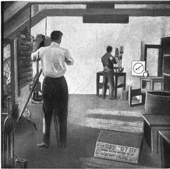
Mr. Frank B. Gilbreth cinematographing a man's work against time, showing the Gilbreth clock.
