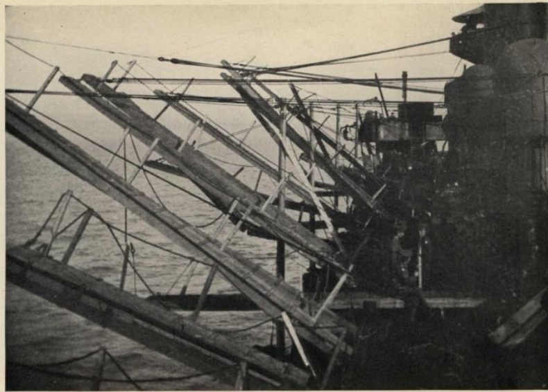
H.M.S. VINDICTIVE'S SPECIALLY CONSTRUCTED GANGWAYS Two of the parapet anchors for grappling the Mole can be seen at the end of the bridge in the background
