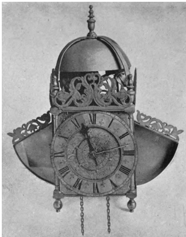
BRASS LANTERN CLOCK, WITH TWO HANDS. Thirty hours; striking and alarum. Anchor pendulum with wings each side and chains and weight below clock. Short pendulum at back. Date, about 1670.
