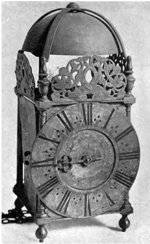
BRASS LANTERN CLOCK, WITH SINGLE HAND. Thirty hours; striking, but no alarum. With chains and weights beneath; short pendulum at back. Date, about 1660. Maker, Daniel Quare (London).
