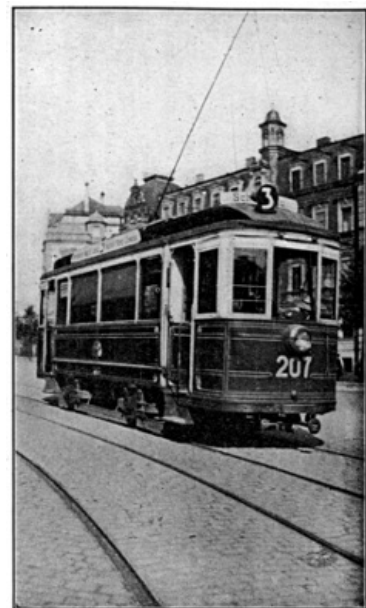
NUREMBERG MUNICIPAL CAR, SHOWING ILLUMINATED ROUTE NUMBER USED FOR EACH LINE.
