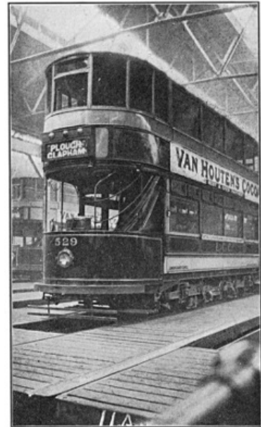
LONDON COUNTY COUNCIL CAR WITH SEVENTY-TWO SEATS. THE SAFEST TYPE IN THE WORLD, WITH THE LATEST MAGNETIC BRAKES AND AUTOMATIC WHEEL GUARDS.
