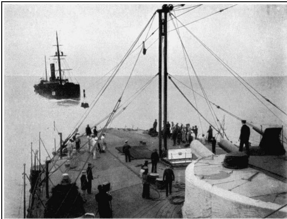
A TEMPERLEY-MILLER MARINE CABLEWAY COALING H.M.S. "TRAFALGAR" AT SEA A carrier, from which are slung the sacks of coal, is hauled backwards and forwards by steel ropes stretching between the foremast of the transport and a mast rigged on the warship.
