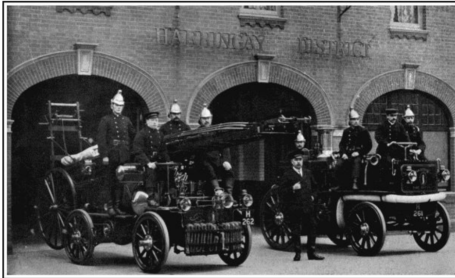
Two Motor Fire-engines built by Messrs. Merryweather, London. That on the left is driven by petrol, and in addition to pumping-gear carries a wheeled fire-escape. That on the right is driven by steam. Both types are much faster than horses, being able to travel at a rate of over 20 miles an hour.
