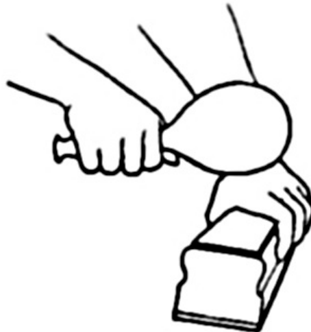
FIG. 15. Proof Planer and Mallet in use
