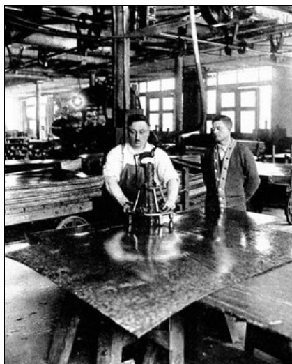
At work on the steel plates for inside finish panels
