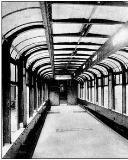
The car ready for the interior fittings. The floor is of monolith construction
