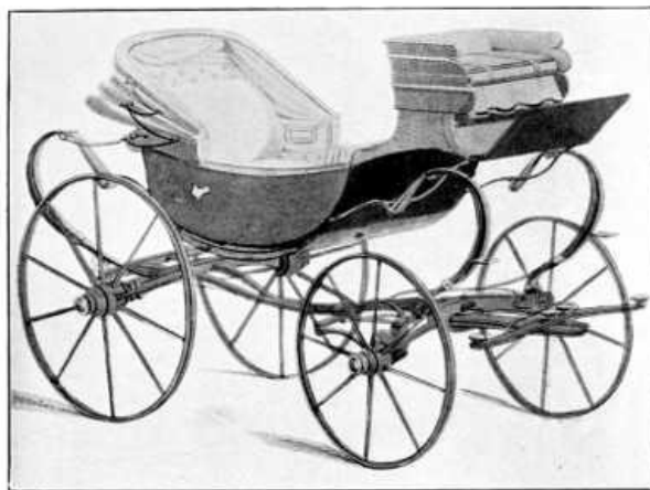
Barouche With Ackerman's Patent Movable Axles
