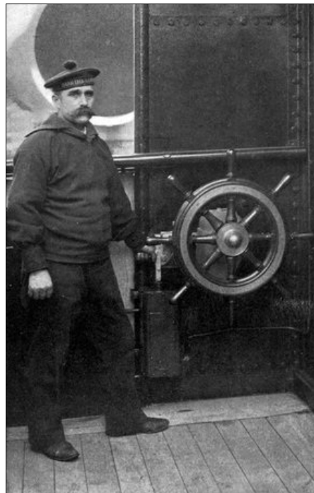
CLOSING, FROM THE BRIDGE, ALL WATERTIGHT DOORS THROUGHOUT THE SHIP BY PULLING A LEVER
