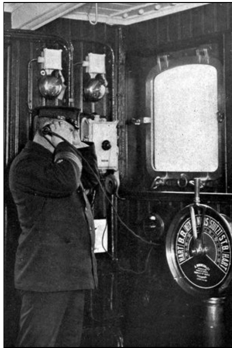
Small dial indicates whether signals come from port or starboard.
