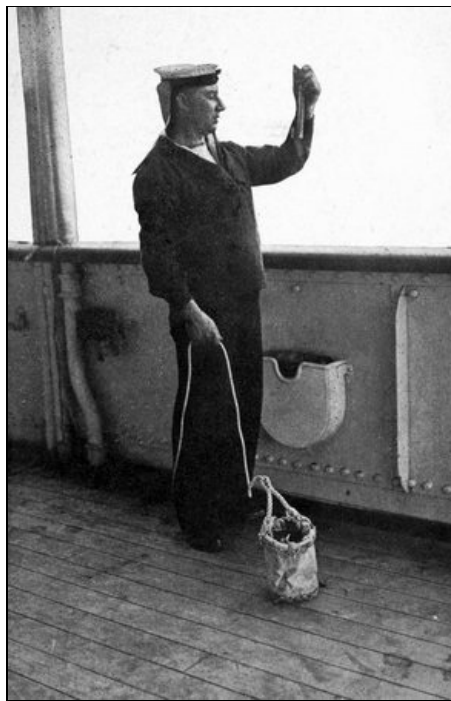
Water is hauled up in the canvas bucket and its temperature taken by thermometer.
