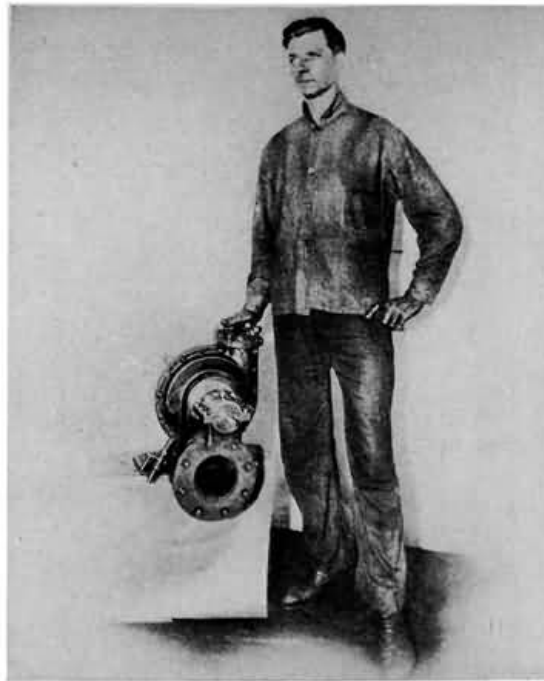
The 200-horsepower engine, which a man could lift with one hand. How the Tesla Turbine compares in size with a man.
