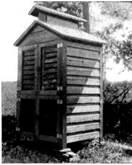
Old-fashioned methods of preserving must again prevail. There is educational value in community conservation. Montclair (New Jersey) boys made community evaporators, having a capacity of from five to eight bushels of fruit a day, at a cost of only $10.
