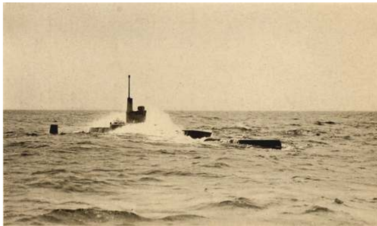
RUSSIAN-LAKE TYPE CRUISING SUBMARINE "KAIMAN" MAKING A SURFACE RUN IN ROUGH WEATHER IN THE GULF OF FINLAND
