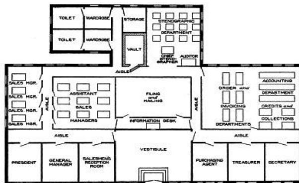
Fig. 10. Floor Plan of a Modern Administrative Building
