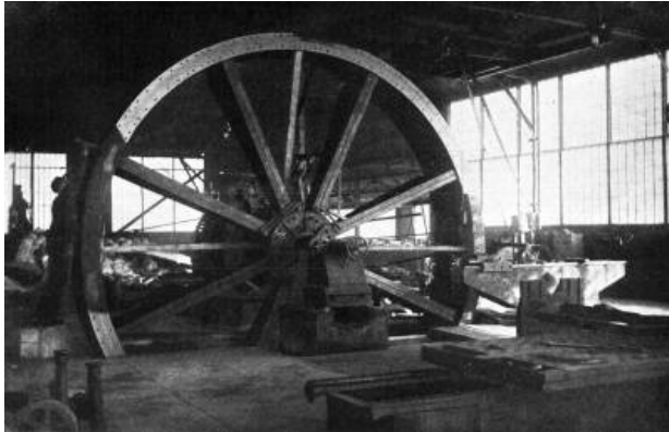
SHOWING USE OF PIT LATHE IN MACHINING A CENTER OF SWING BRIDGE Chicago Bridge & Iron Works, Chicago, Ill.
