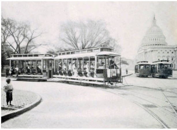
FIG. 28.—VIEW OF STREET RAILWAY LINES IN WASHINGTON OPERATED BY UNDERGROUND CONDUCTOR OF TYPE SHOWN IN FIG. 27.
