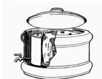
FIG. 62. Water cooler containing water tank.
