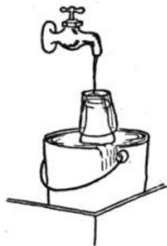
FIG. 61. Cooling with running water.
