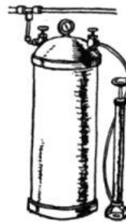
FIG. 157. Pressure tank for gas.
