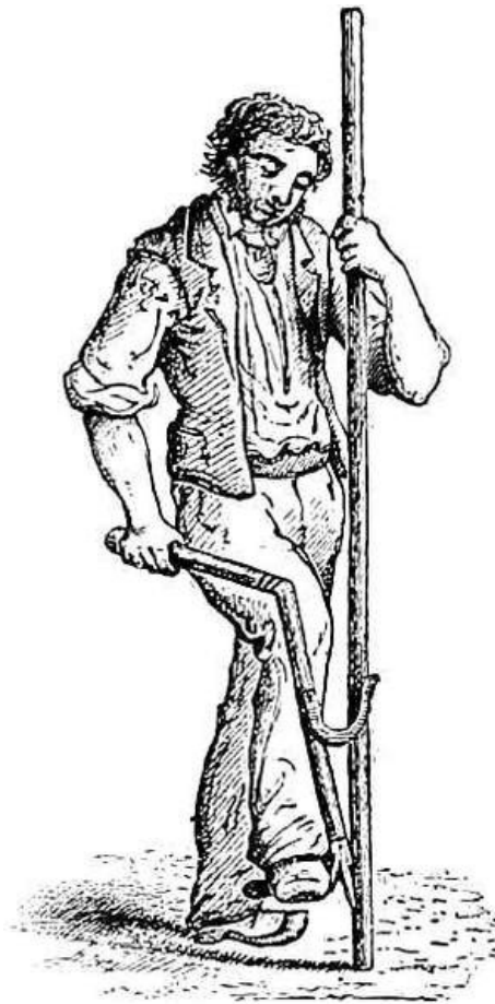
APPARATUS FOR FIXING VINE-STAKES.
