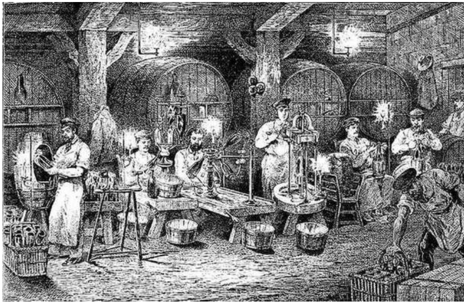
THE DISGORING, LIQUEURING, CORKING, STRINGING, AND WIRING OF CHAMPAGNE.
