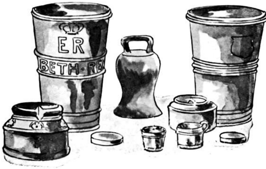
FIG. 57.—OLD MEASURES BASED ON THE WINCHESTER STANDARD. ( Sketched by permission of the Corporation of the City of Winchester. )
