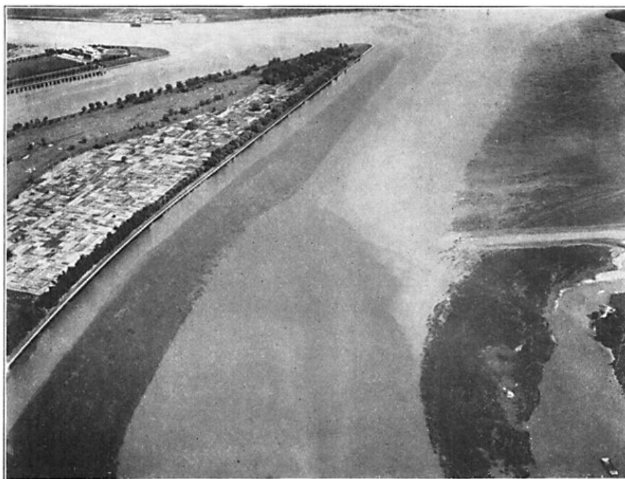
THE BED OF POTOMAC RIVER, AT WASHINGTON. From an altitude of a few hundred or a few thousand feet, submarine features are clearly revealed to great depths. Objects have thus been photographed 45 feet under water. The shoals are submerged to a depth of from 2 to 5 feet. In favorable weather, aerial photographs are valuable in making hydrographic surveys. ( Photographed from the air by Dr. W. T. Lee, U. S. Geological Survey. )
