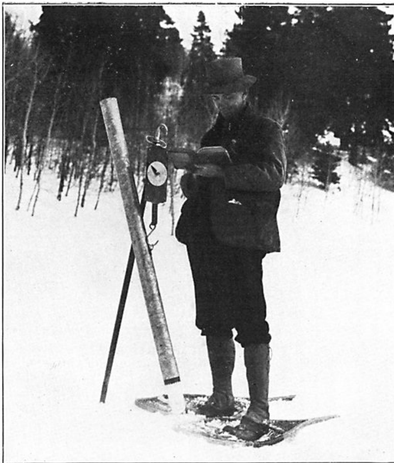
A SNOW SURVEYOR AT WORK. Note the cylindrical snow sampler, with its serrated cutting edge, and spring balance for weighing the sample of snow ( Photographed by J. C. Aller. )
